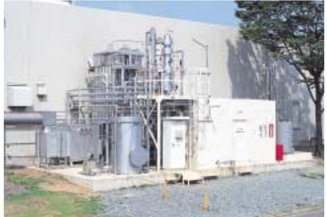
Dichloromethane recovery plant (Kofu Factory)
